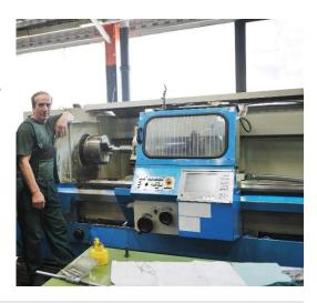
**OSHA Standard 1910.212(a)(1)** One or more methods of machine guarding shall be provided to protect the operator and other employees in the machine area from hazards such as those created by point of operation, ingoing nip points, rotating parts, flying chips and sparks.
