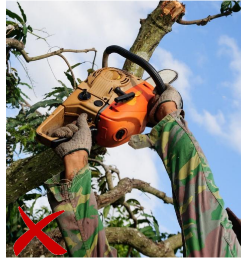
Do not use a chainsaw to cut directly overhead.
